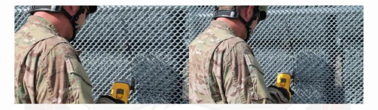
IFI 9 Gauge 3/8" Weave Chain Link | One-person attack utilizing 36V battery operated grinder Description: This test involved one-person cutting through 9 Gauge 3/8" weave chain link fence. The attacker cut a vertical line large enough to allow passage of a person through the fence. The test started when the grinder first touched the fence, and ended when the attacker was successfully through the opening.
