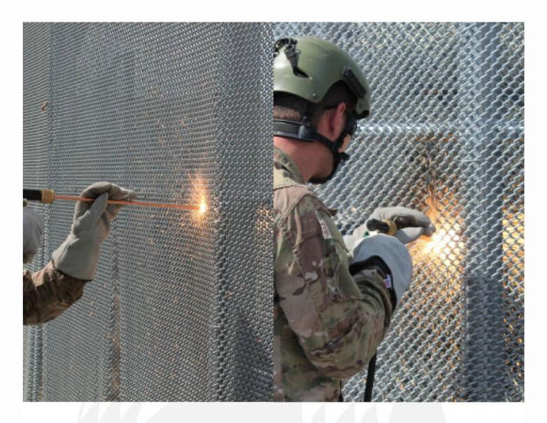
IFI-6 Extreme Cut 6 Gauge 5/8" Weave Chain Link | One-person attack utilizing Broco Torch Description: This was a one-person attack utilizing a Broco Torch against IFI 6 gauge 5/8" chain link weave. The attacker used the torch to create a vertical opening in the fence, which was then cooled with water before penetration. The test started immediately after the torch was lit and ended when the attacker was successfully through the opening.
