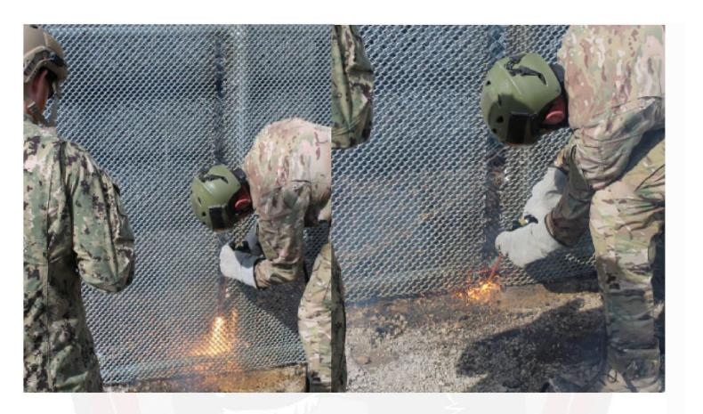
IFI 9 Gauge3/8" Weave Chain Link | One-person attack utilizing Broco Torch
